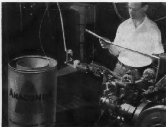
PAY-OFF BARRELS with big coils of brass wire cut down-time 90% at wire forming machines for West Haven (Conn.) Buckle Co. Machines making surgical buckles had used light coils for free pay-off; new coils had to be fed in about every hour.
